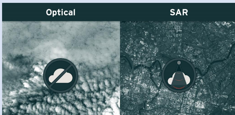
Fig: Difference between optical remote sensing systems and Synthetic Aperture Radar (SAR) (Source: ursaspace.com)
